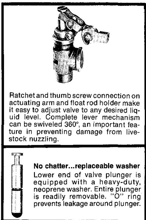
Ratchet and thumb screw connection on actuating arm and float rod holder make it easy to adjust valve to any desired liquid level. Complete lever mechanism can be swiveled 360°, an important feature in preventing damage from livestock nuzzling.
