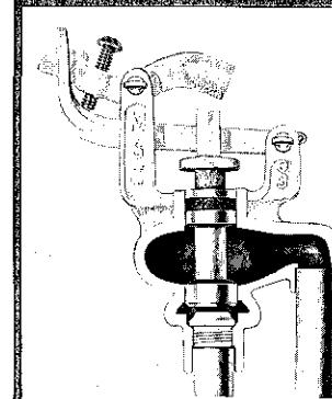
Cutaway shows how compound lever action works in conjunction with plunger, plunger seat and valve seat to provide positive opening and closing at all pressures. Also, note by-pass design of water passage that quiets flow.
