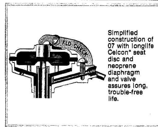
Simplified construction of 07 with longlife Celcon\* seat disc and neoprene diaphragm and valve assures long, trouble-free life.
